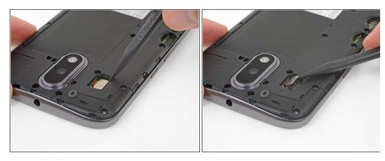
• Use a spudger to disconnect the camera flash connector by prying it straight up.
