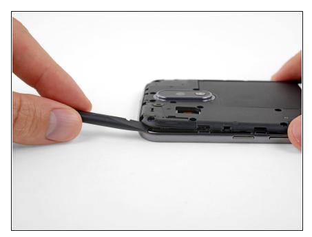
Insert a spudger under the midframe at the top left corner, and gently twist to separate it from the body of the phone.
