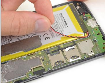
Peel off any tape securing the battery wires, and then push the battery wires towards the battery to de-route them from the black bracket on the motherboard.
