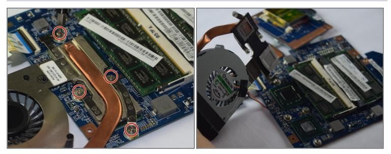
• Remove the four (4) screws that are holding the CPU's cover on
