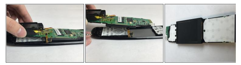
• Carefully remove the motherboard from the top piece of the case.
