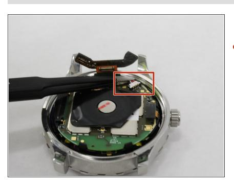
Utilize tweezers to pull the white battery connector from the motherboard.
