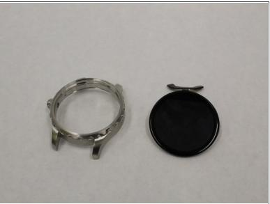
• The screen can now be removed out of the front-side of the watch.
