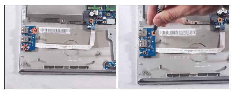
• Use a JIS #0 screwdriver to unscrew the two 4mm screws from the board.
