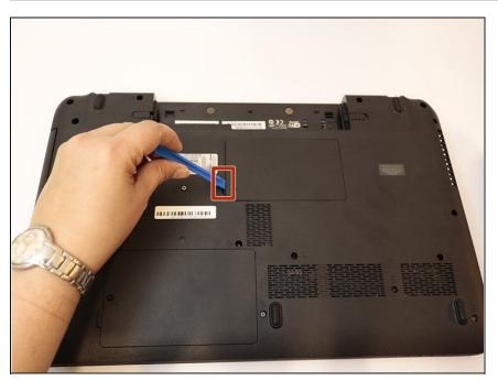
Use the plastic opening tool to pry open the CMOS battery cover. Wedge the prying tool in, beginning at the indent in the cover.
