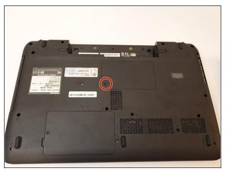
Use the Phillips #1 screwdriver to remove the one 4.6 mm screw holding on the cover located on the bottom center of the laptop.
