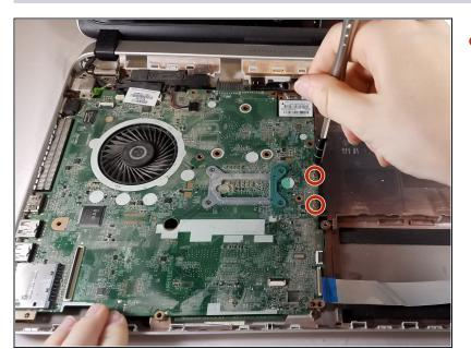
Remove the two 5.66mm screws from the motherboard using Phillips head screwdriver J0
