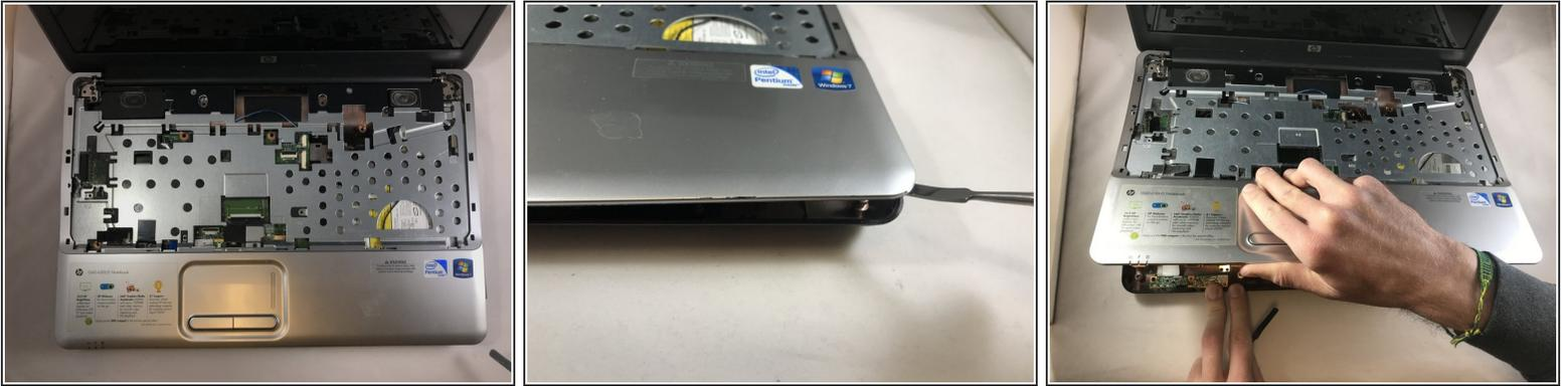
**i** In order to be able to unplug the cables that connect the screen to the motherboard, we will need to remove the metal support.
