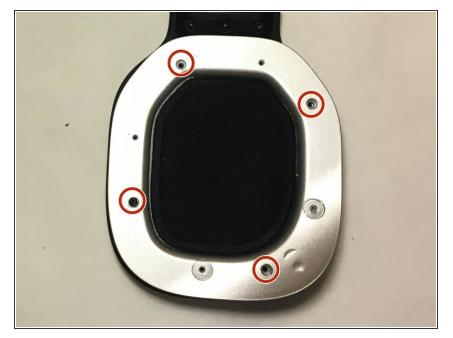
Remove the four 3.5mm Phillips head screws circled in red and remove the silver cover.
