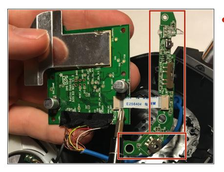
Separate the secondary mother board from the motherboard by pulling firmly to the right on the white connector.
