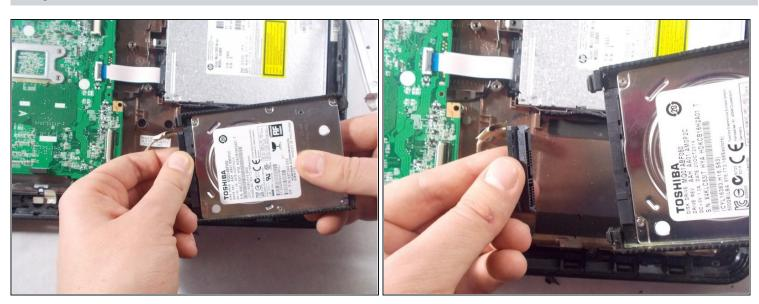
Remove the connection from the left of the hard drive connecting it to the rest of the laptop and remove the hard drive from the laptop.
