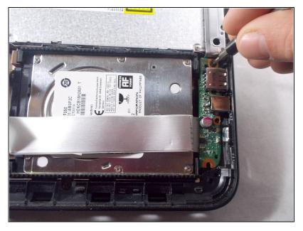
After removing the battery and palm rest, unscrew the two 3 mm PH1 Phillips head screws that hold the small tab that secures the connection of the USB port and headphone jack.
