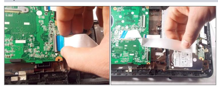
Pull the connected cord out of the previously lifted tab and remove from laptop.
