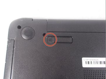
Slide the left switch to the right so that the icon of a locked padlock is no longer visible and the icon of an unlocked padlock is now visible.
