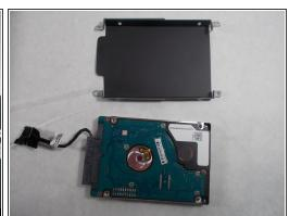
Remove the 4 screws from the hard drive bracket and separate it from the hard drive.
