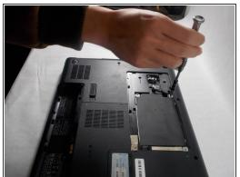
Use a screwdriver to remove the three Phillips PM3.0x4.0 screws on the hard drive.
