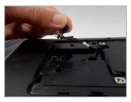
Disconnect the hard drive cable from the system board and gently remove the hard drive.
