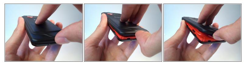
Press your thumbnail into the slot between the rear panel and the front case located in the bottom of the phone.
