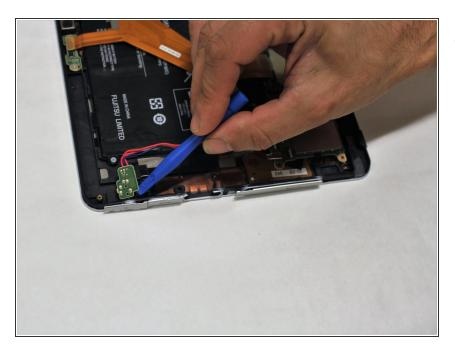
Pry the AC power port board away from the device.
