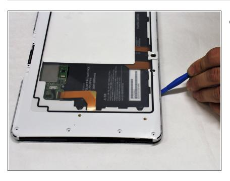
Gently slide the plastic opening tool along the entire seam popping the clips free.
