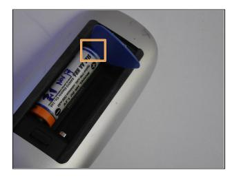
Make it lever to the other battery with the same technique of the battery compartment.
