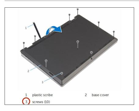
Remove the ten screws that secure the base cover to the base of the computer.
