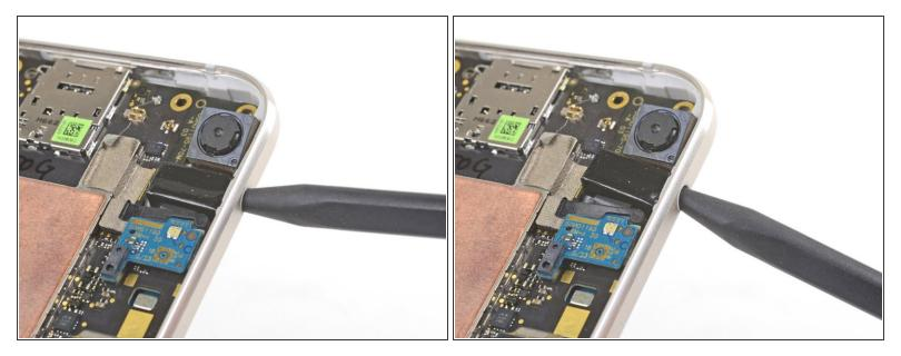
Insert the point of a spudger into the headphone jack port and pry upwards to loosen the port from its socket.
