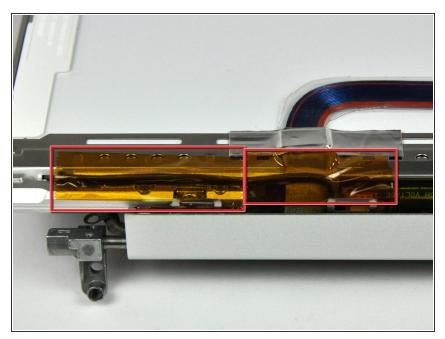
(i) If necessary, remove the two pieces of tape covering the inverter leads.
