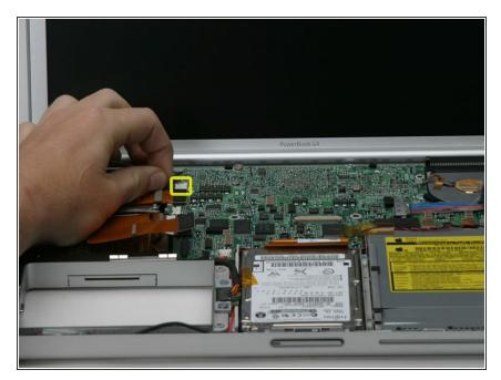
• Disconnect the inverter cable from the logic board.
