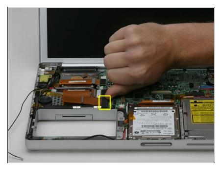
• Disconnect the large orange Airport ribbon from the logic board.
