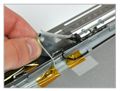
• Lift the antenna board out of the clutch cover.
