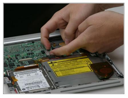
Remove the two pieces of orange tape covering the display data cable and disconnect the cable from the logic board.
