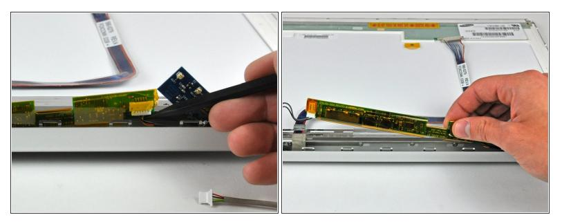
The inverter is an extremely thin circuit board that is very delicate and easily cracked. Take care when handling.
