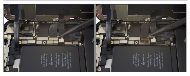
Use the point of a spudger or a fingernail to disconnect the OLED panel cable connector.
