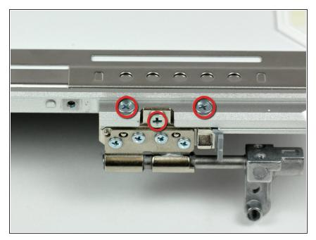
Remove the three Phillips screws securing the left clutch hinge to the front bezel.
