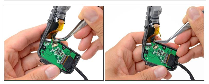
Using your fingers or tweezers, gently pull out the backlight ribbon cable from its connector on the button board.
