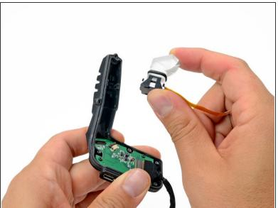
Remove the viewfinder lens assembly from the viewfinder housing.
