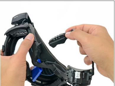
Remove the viewfinder assembly by pulling it through the opening in the top of the frame.
