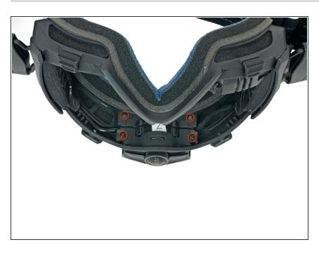
Remove the four 7.1 mm Phillips screws securing the camera housing to the goggle frame.
