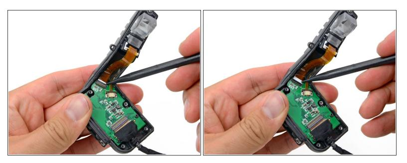
• Use the tip of a spudger to flip up the retaining flap on the LCD ribbon cable ZIF connector.
