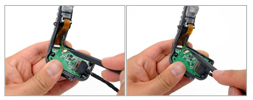
Use the tip of a spudger to push out the retaining clip on the viewfinder backlight ribbon cable ZIF connector.
