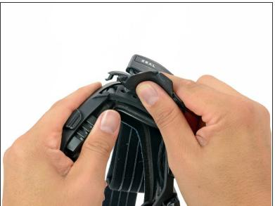
Once the bottom is free, continue pulling to free the bottom of the strap mount cover from the frame.
