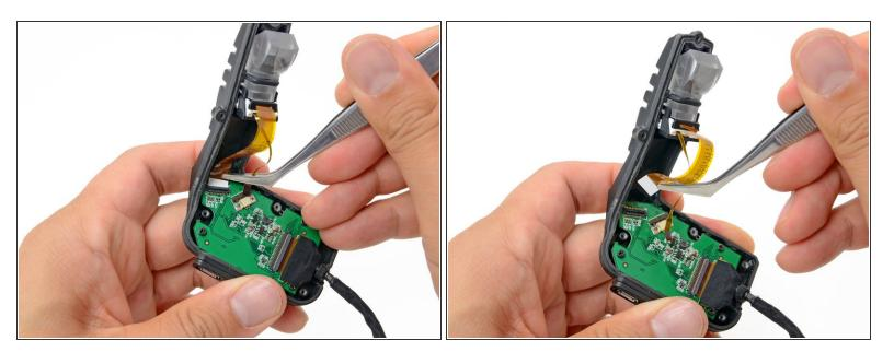
Using your fingers or tweezers, remove the LCD ribbon cable from its connector on the button board.
