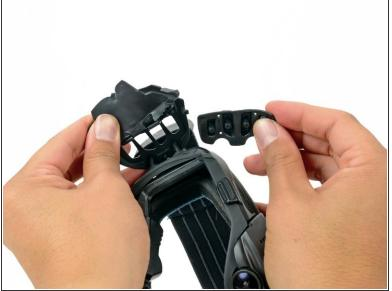
Hold the strap mount cover away from the frame and remove the keypad.
