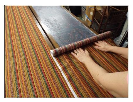
Lay the screen on a table or some saw horses and roll the fabric onto the screen.
