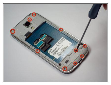
Remove the ten 4.0 mm screws on the back of the phone using the #00 Phillips screwdriver.
