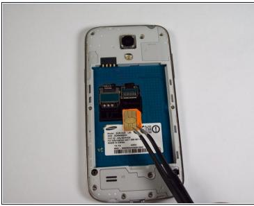
• Using tweezers, remove the SIM card by sliding it towards the bottom of the device.
