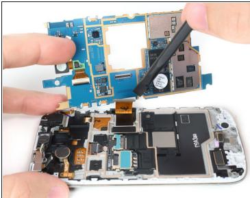
• Put the flat end of a nylon spudger under the lip of the digitizer press-fit connector and lift up to release the connector and free the motherboard.
