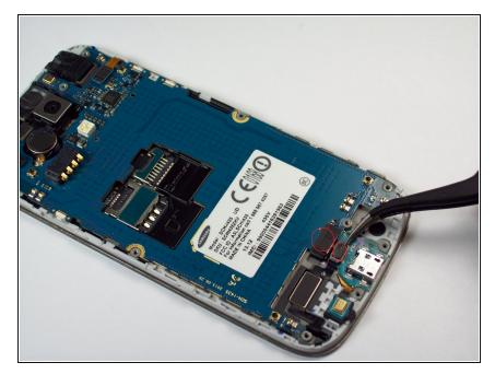
Use a pair of tweezers to lift the two charging assembly press fit connectors free.
