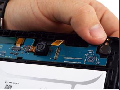
Use a spudger to lift up and release the press-fit display cable connector from the motherboard.
