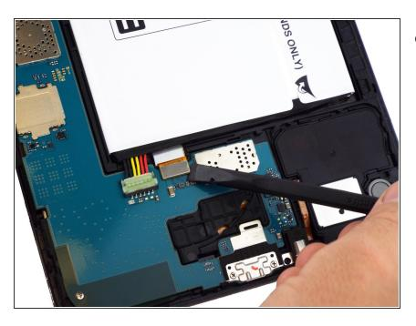
Use the flat end of a spudger to lift up and disconnect the LCD screen press-fit connector.
