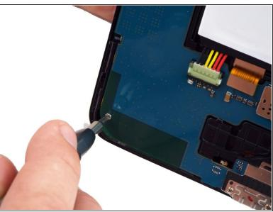
Use a PH000 screwdriver to remove the two 3 mm screws on the left side of the motherboard.
