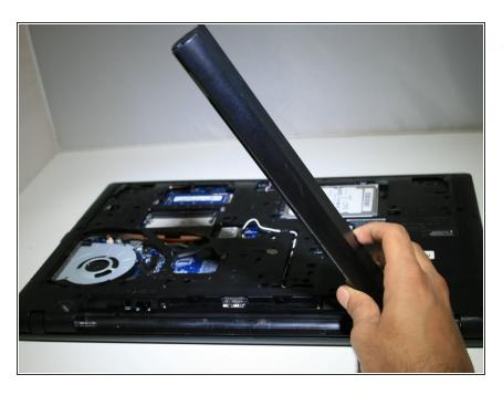
Remove the battery from the device.
