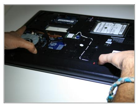
Press along the opposite side to release the battery from the Laptop then remove.
