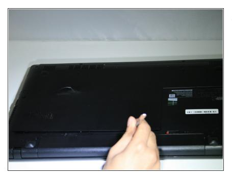
Use a spudger to lift the back cover and remove it from the device.
