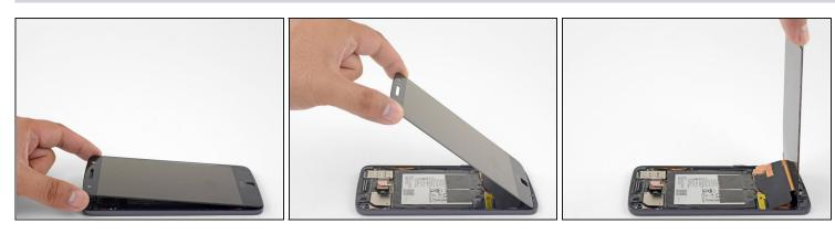
• Lift the earpiece end of the display up to provide access to the display cables.
