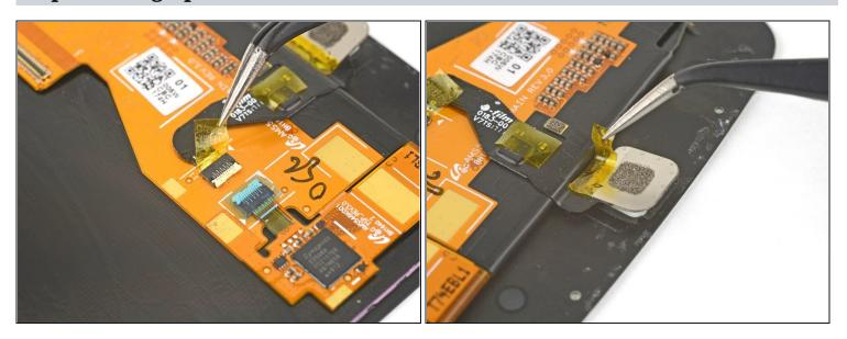
• Use <u>tweezers</u> to peel off any tape on the home button connector and home button
