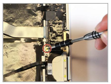
Remove the gold 2.0mm corner screw by turning it counterclockwise with a T3 Torx screwdriver.
