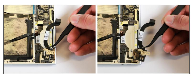
Use the needle-nose tweezers to remove the charging port by lifting the component up and out of the Pixelbook.
