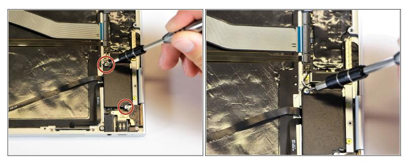
Remove the two 3.0mm silver screws from the thin, black component by using a T3 Torx screwdriver to turn the screws counterclockwise.
