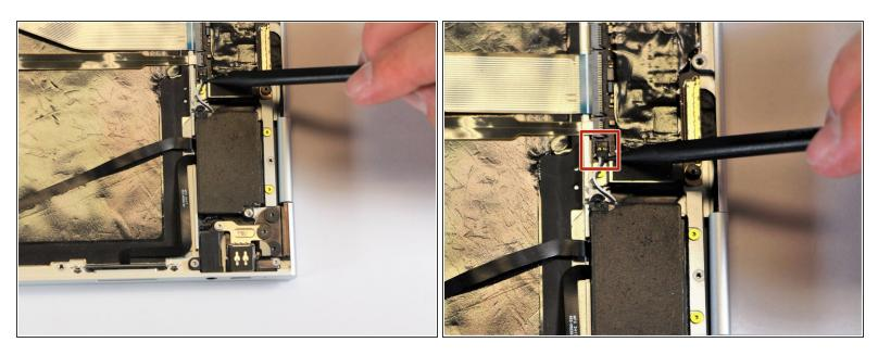
Disconnect the thin, black and white cord from the motherboard by using the spudger to snap the connector up and out of place.
