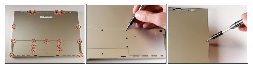
Remove the seventeen 3.0mm T5 Torx screws from the bottom panel.
