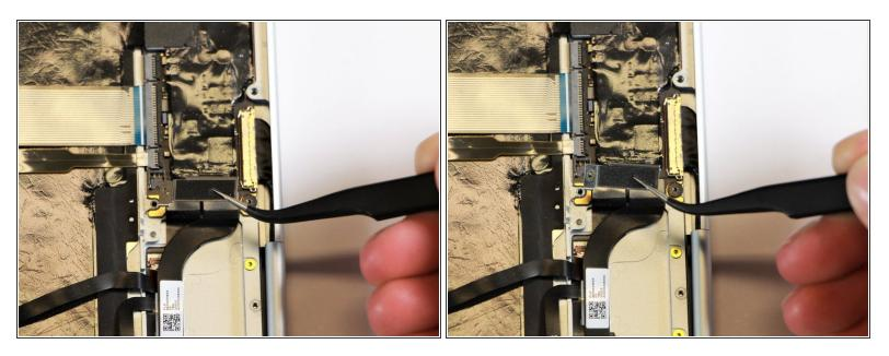
• Using needle-nose tweezers, remove the silver casing by lifting it up and out of the computer.
