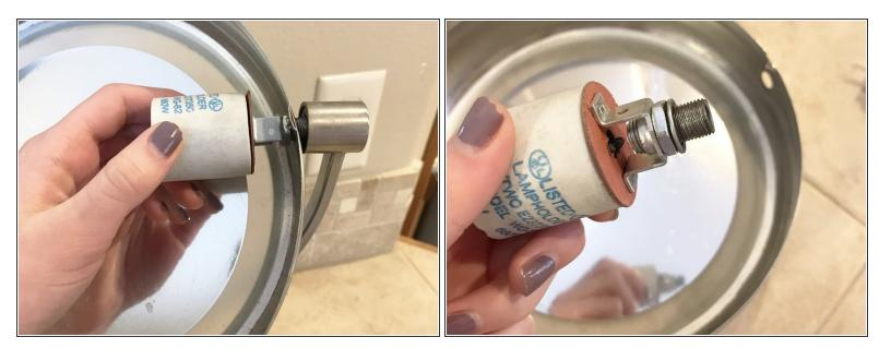
• Remove the larger bolt on the opposite side by twisting it counter-clockwise.
