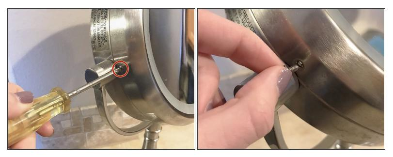
Using the Phillips head screwdriver, unscrew the screw on the side of the mirror.
