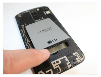
Remove the battery from the phone by lifting up on the bottom end of the battery.
