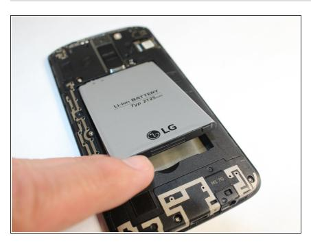
Remove the battery from the phone by lifting up on the bottom end of the battery.
