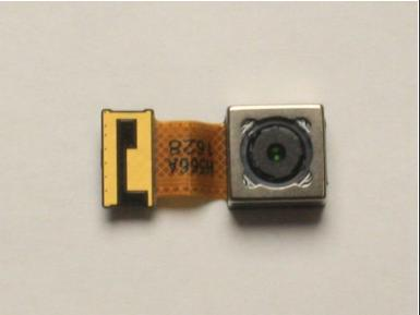
Pull up on the gold film-like connector which is to the left side of camera. Once you have pulled the connector loose you can then gently lift the rear camera out of the phone. To reassemble your device, follow these instructions in reverse order.
