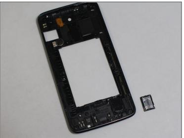
• Use the <u>tweezers</u> to lift the loudspeaker out of place.
