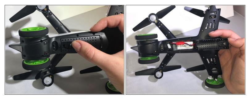
• Pull down the battery cover on the bottom of the drone and open it.
