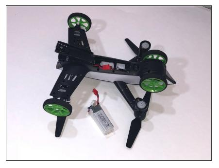
• Remove the battery from the device.
