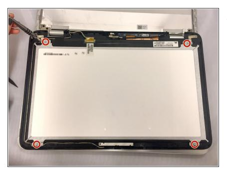
Remove the four 3mm screws using the Phillips #00 screwdriver.
