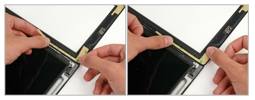
Place the remaining thin L-shaped adhesive strip on the top right corner of the front panel, near the camera mounting bracket.
