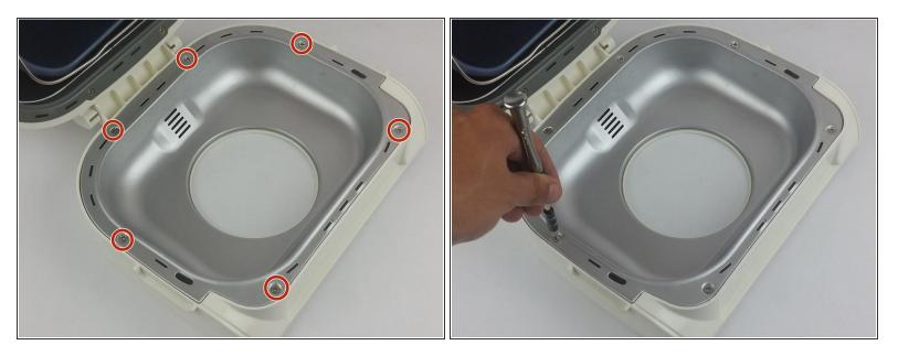
• Remove the six 55.4mm Phillips #1 screws from the top panel.
