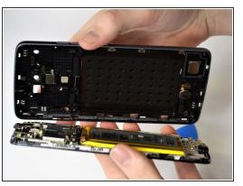
• Use a plastic opening pick between the screen and side trim battery cover to remove the screen.
