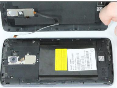
After removal of the two 3.4mm JIS 00 screws, disconnect the connector that attaches the ribbon wire from the main part of the phone.
