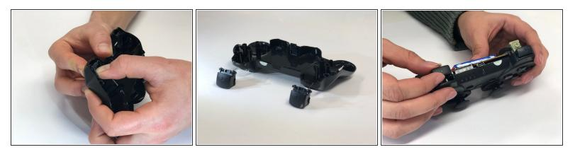
• Remove the left and right bumper buttons (L1, L2, R1 and R2).
