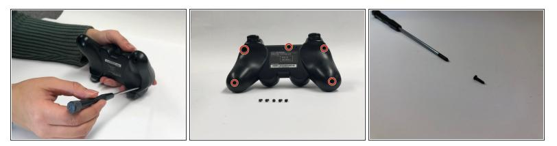
• Remove the five 7.2 mm Phillips screws at the back of the controller.
