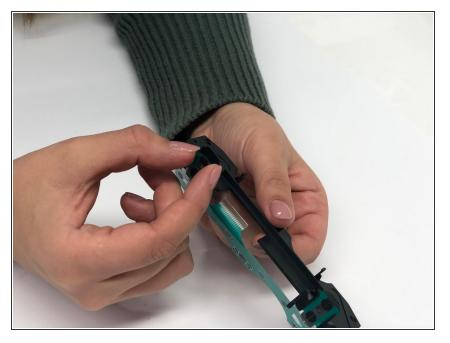
Remove the thin flexible green PCB by lifting and pushing the two outer flaps.
