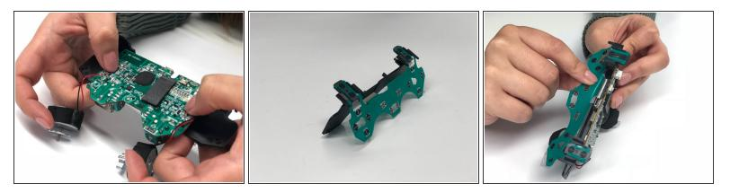
Remove the thin flexible green PCB by pulling out the black plastic circuit board cover, relatively in the middle the motherboard (the hard PCB) and by pressing click fingers on top of the motherboard.
