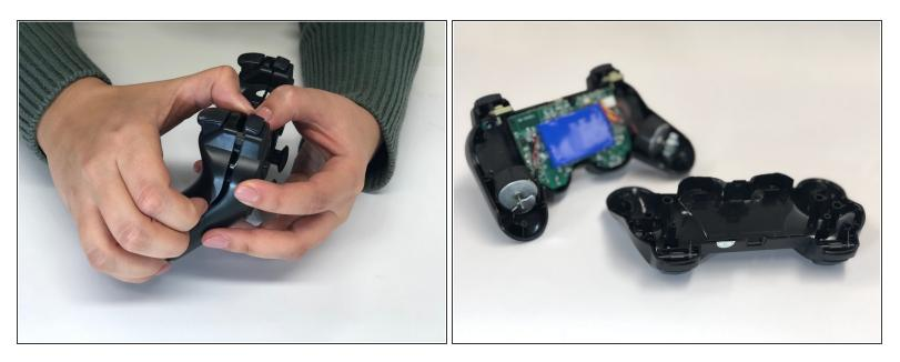
• Separate the bottom case from the upper part. All the electronics stay in the upper part.
