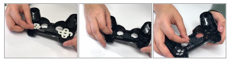
Remove all loose parts from the body. (Consisting of white rubber button underlays, black plastic buttons and a black rubber underlay for the start and select button.)
