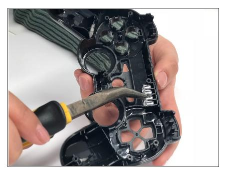
Remove the transparent plastic part covering the LED-lights by taking it out with a pair of pliers.
