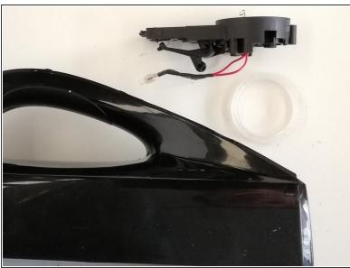
Remove the silicone ring from the hole in which the heating element was placed. It can be easily removed by pulling on it.
