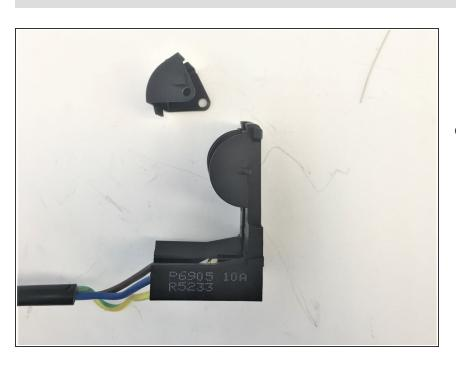
Remove the hood of the electrical subassembly by pulling on one side of the hood to release the snapfit hinge.
