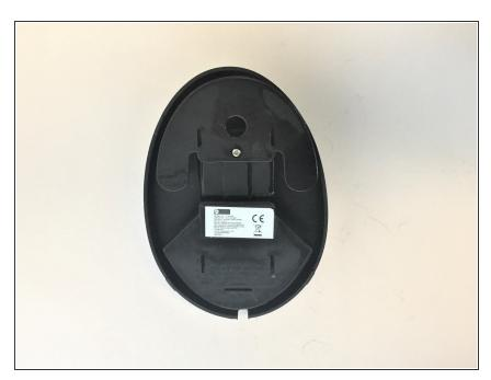
Using the three-winged screwdriver, remove the three-winged screw from the bottom of the hot plate.
