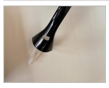
Remove the on/off switch by pulling apart the snap fits and sliding the switch out of the hole in the handle.
