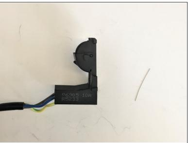
Remove the wire spring from the electrical subassembly by sliding it out of the hook on the hinge and pulling it of the subassembly.
