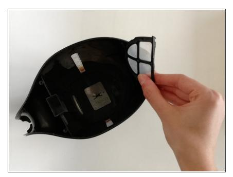
Remove the filter from the kettle by pulling up on it in order to slide it out of the tracks it is in.
