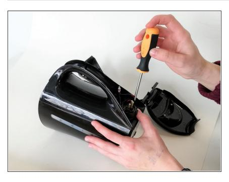
Using the Phillips head screwdriver, unscrew the three Phillips head screws in the handle.
