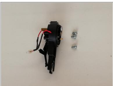
Pull the electronic part out of the kettle.
