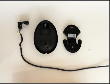
Remove the electrical subassembly from the base of the hot plate; it will lift out with no resistance.
