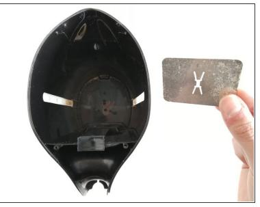
Remove the metal plate from the bottom of the inside of the kettle by pulling up on it to release it from its snapfit.
