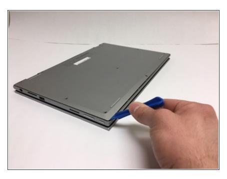
Insert a plastic opening and run it along the edge of the back cover.
