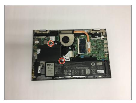
Unscrew and remove the 2 of the 3mm Phillips head screws holding the hard drive in place.
