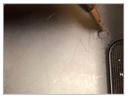
First turn over your computer and remove all of the rubber stoppers on the back.
