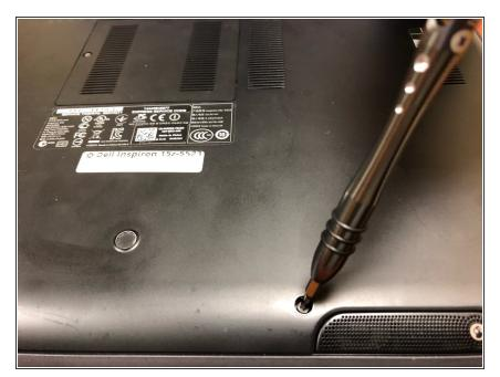
• Then remove all the screws that were under the rubber stoppers.
