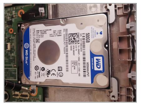
Remove the three screws from the hard drive and remove by pulling straight out.
