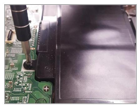
• Remove the battery by unscrewing the 5 screws and pull straight out.
