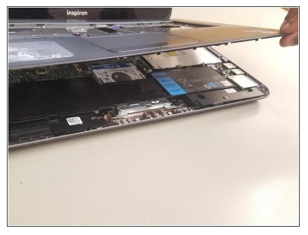
• Take screw out of the surface below the keyboard and remove the top layer of the computer off of the base.
