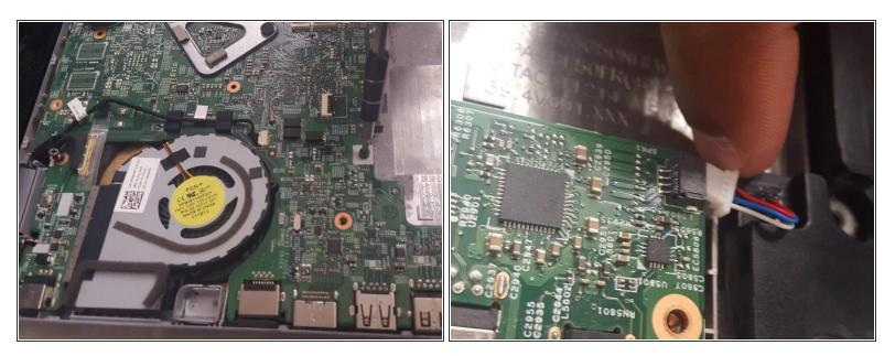
• Unscrew motherboard and remove the two clips.
