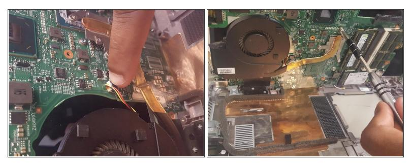
• Flip motherboard up, unscrew the three screws, and unclip the fan.
