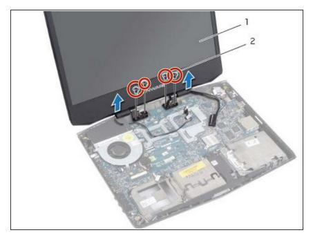
Replace the screws that secure the display assembly to the computer base.
