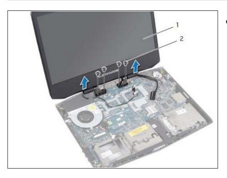
Align the screw holes on the NEW display assembly with the screw holes on the computer base.
