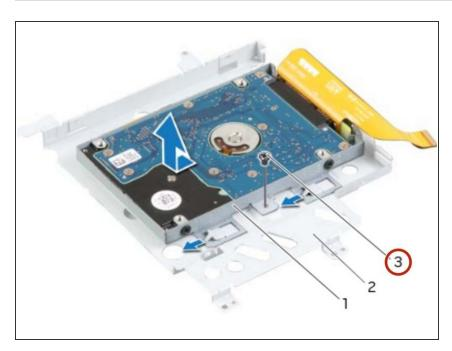
Align the screw hole on the secondary hard-drive assembly with the screw hole on the main bracket.
