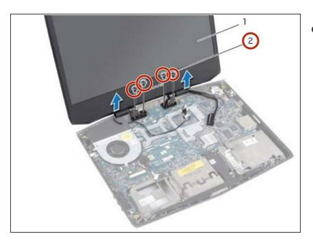
Remove the screws that secure the display assembly to the computer base.
