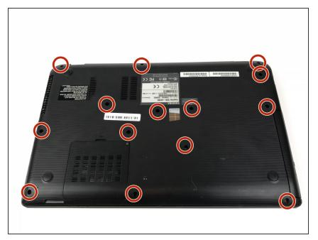
Remove the fourteen 5mm Phillips #0 screws from the bottom of the laptop.
