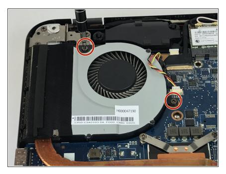
Remove the two 5mm Phillips #0 screws from the fan.
