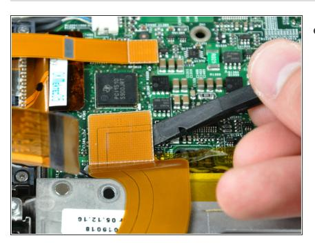
Use the flat end of a spudger to pry the sound card cable connector up off the logic board.
