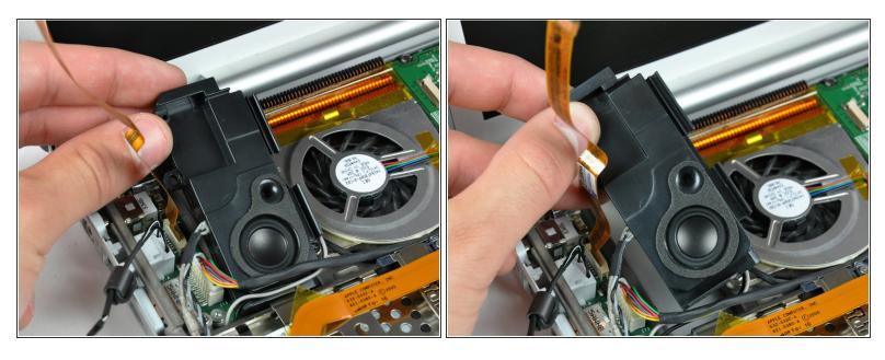
• Lift the left speaker from its rear edge and maneuver it out of the lower case, minding the cables sitting in the channel near the front edge of the left speaker.
