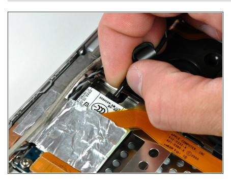
Disconnect the RJ-11 cable from the modem.
