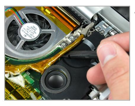
Use a spudger to de-route the display data cable from the channel in the right speaker.
