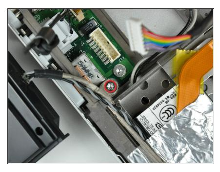
Remove the single 6.9 mm T8 Torx screw securing the speaker cable ground loop to the lower case.
