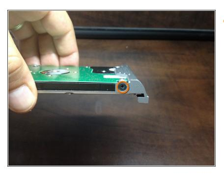
The hard drive bezel is attached by two 3.5mm #1 Phillips screws.
