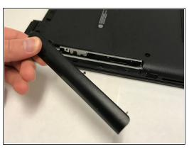
Locate the CD Compartment panel and gently slide it out.
