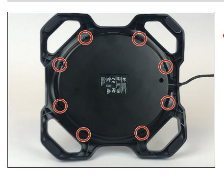
Remove the eight 10mm Phillips #1 screws from the bottom.
