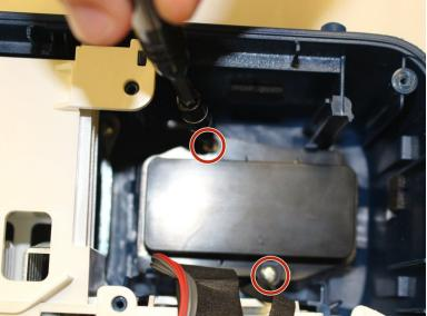
Unscrew the PH 1 (10 mm) screws from the black outer casing of the auxiliary port.
