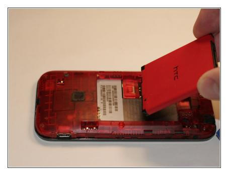
Remove the red battery to replace.
