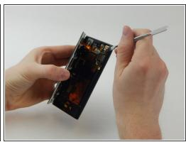
Wedge a spudger underneath the silver rectangle in the upper right corner until it pops off the back of the phone.
