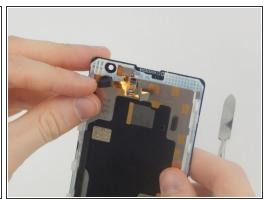
Wedge a spudger underneath front-facing camera on the upper left corner of the screen. Pry
