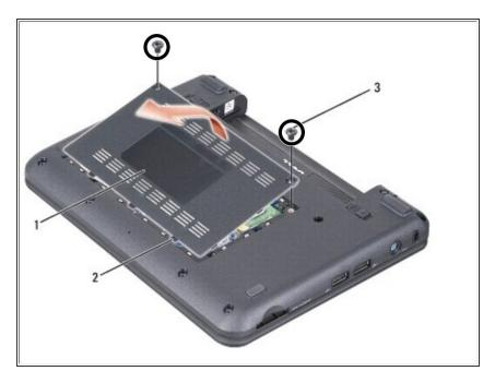
Remove the two screws on the module cover.
