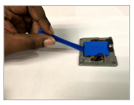
Remove the speakers battery from its metal base, utilizing the plastic opening tool.
